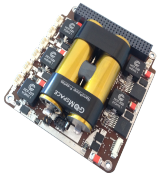
Electrical Power System
